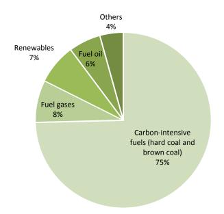
**Figure 1.** The structure of usage of fuels used to heat production in 2015 Source: Author's own elaboration based on: Raport Prezesa URE – Energetyka cieplna w liczbach – 2015, 2016:13
