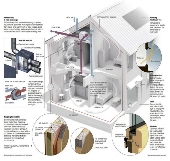
Figure 4. Technologies used in a passive house
