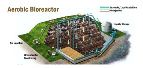
Figure 4. Aerobic solid waste bioreactor landfill
