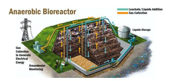
Figure 3. Anaerobic solid waste bioreactor landfill
