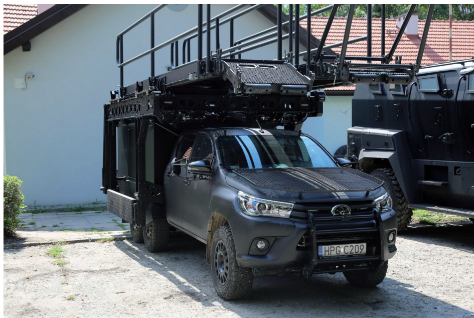
Photo 2. Assault platform based on the Toyota Hilum car - front view
