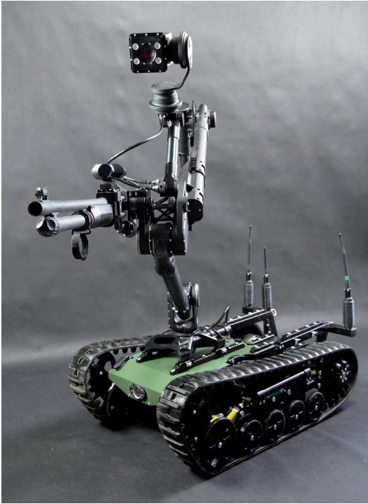
Photo 1. Modern Piap Patrol robot used to detect CBRN threats
